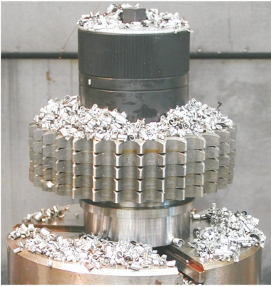
Clamp nut clamping sprockets during milling
