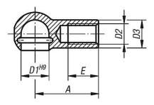
Form B with snap ring and groove for circlip
