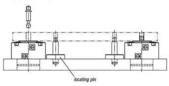
Simultaneous clamping and positioning of a workpiece
