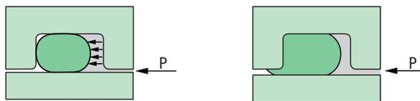
The reference values given in the table for gap dimensions for standard elastomer are maximum values based on central alignment of the components. The permissible values for the sealing gap are dependent on pressure, material hardness and diameter. All specifications are based on experience and should only be regarded as guideline values.
