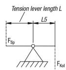
Effective clamping force  $F_{\text{Kol}}$  is dependent on piston force  $F_{\text{Kol}}$  and tension lever length L
