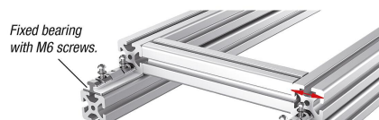
Fixed bearing with M6 screws. Floating bearing with M5 screws. The profiles can move laterally to each other.
