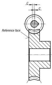
For lateral mounting of the worm wheel, the toleranced reference face is decisive. The lateral tolerance "c" must not exceed 0.15 mm for all centre distances.
