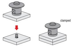
Press the latch over the clamping pin without pressing the knob. The latch is now locked.
